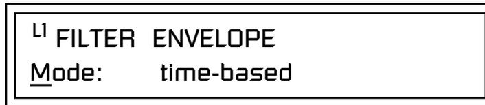
3. Turn the **data entry control** clockwise. The Mode field will change to Repeat as shown below.
