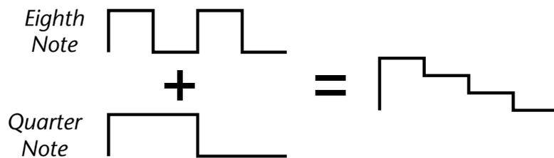
Adding these two clocks together in equal amounts produces a stairstep waveform.
