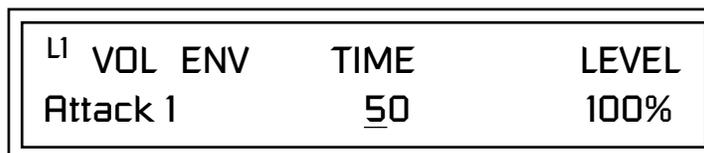
3. Increase the Attack 1 time value and play a note. The attack controls the time it takes for the sound to reach the Attack level when a key is pressed and held.
