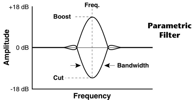
The parametric filter is quite flexible. Any range of frequencies can be either amplified or attenuated. Several parametric sections are often cascaded in order to create complex filter response curves.
