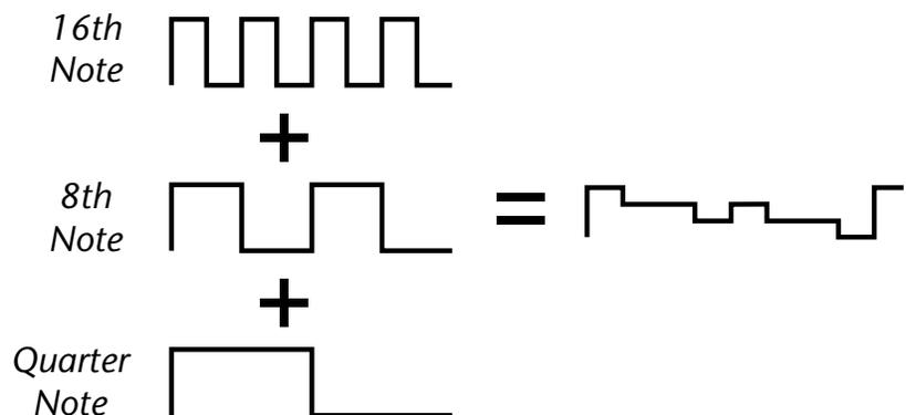
Adding multiple clocks with unequal amounts produces complex repeating patterns.
